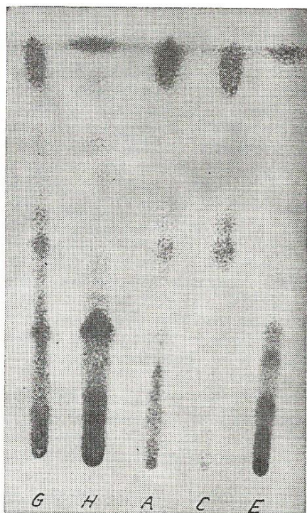
Fig. 2 — Thin layer chromatography of fractions G, H, A, C, E extracted from propolis
